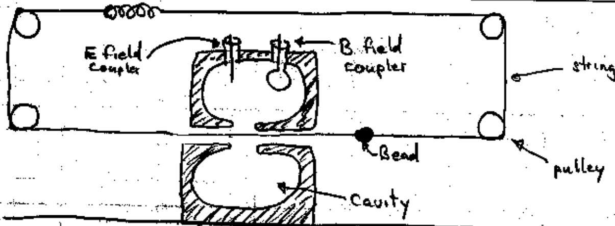
The cavity has two couplers. One is a quasi-B field coupler in which the angle of the coupling loop with respect to the magnetic field can be changed in order to change the coupling. The other coupler is a E field coupler that is weakly coupled to the cavity.
